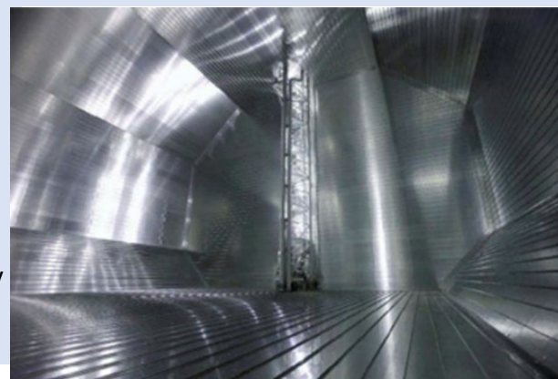
Figure 5 Inside of a membrane tank of a ship (Bruce & Eyres, 2012)
