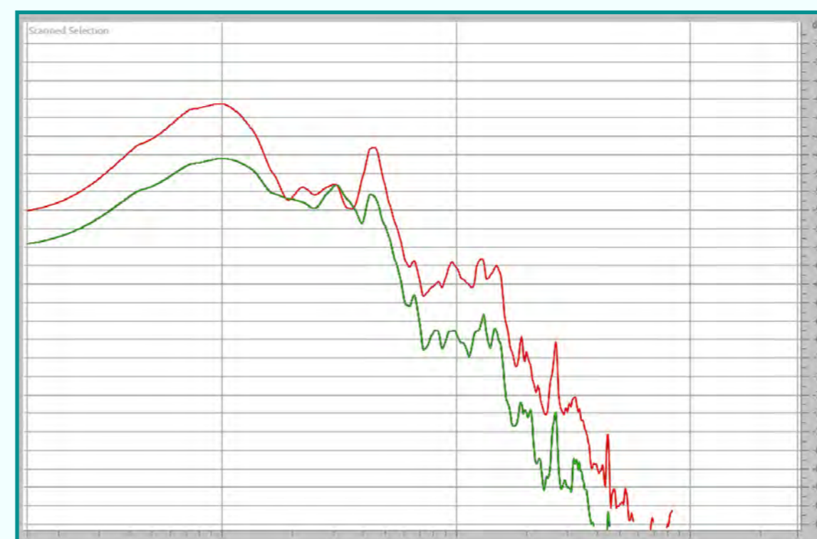
Figure 5 - Low Speed Driving Pre vs Post Treatment Frequency Response
