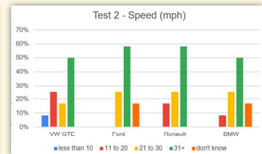
Graph 4: Answers from 12 participants as to how fast the vehicle was travelling. All vehicles were travelling at 15m/s (33 mph).
