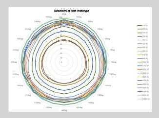
The prototype source does not fall in the requirements set by ISO 3382-1:2009. When measured, the source used a basic pink noise file with no alterations to the equalisation. The deviance is around ±2dB where it should be ±1dB. The drivers used were not checked to be equal in performance before the source was put together.
