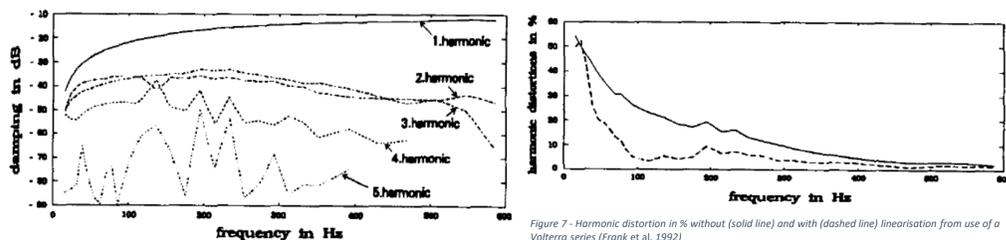
Figure 6 - Harmonic distortions of a moving coil loudspeaker
