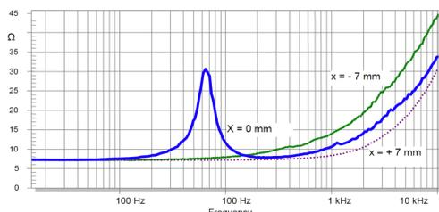
Figure 3 - Input electrical impedance of a moving coil loudspeaker free floating and clamped at +/- 7mm (Klippel 2005a)
