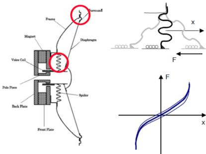
Figure 5 - Suspension system in a typical moving coil loudspeaker and force reflection curve (Klippel 2005a)
