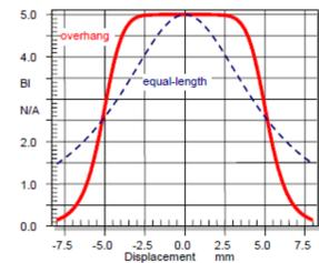
Figure 1 - Force factor versus coil displacement for a loudspeaker with an overhang motor arrangement and an equal length arrangement (Klippel 2005a)
