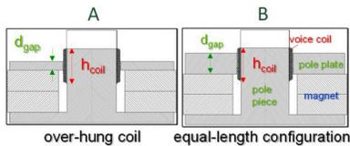
Figure 2 - Typical motor arrangements with an overhang configuration and an equal length configuration (Klippel 2017)
