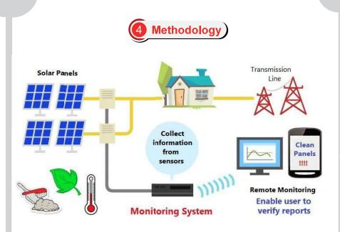
Panel voltage decreases with the increasing in temperature. Therefore, the cooling operation (fan)needs to be started in order to compensate with the loss of efficiency.
