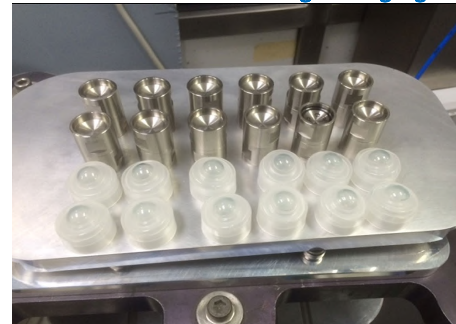
Successful demould using testing rig
