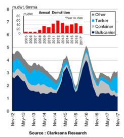
The graph shows the six month moving average of global monthly demolition volumes in dwt terms over the last 5 years, split by vessel sector. The bars on the inset graph show total historical annual demolition in dwt. A wide range of demolition data is available on the *Shipping Intelligence Network*.
