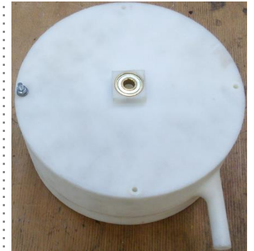
A water turbine printed by AM
